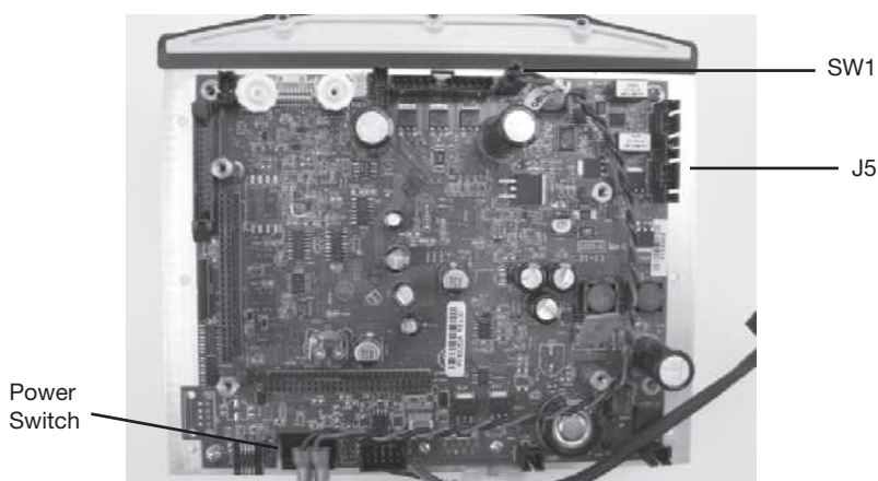
Figure 5.8 Main Control Board (MCB)
